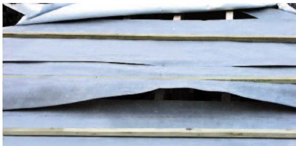
The results from the test method now enable any underlay to be categorised into use by zone (1-5) across the country for the given batten gauge tested.
